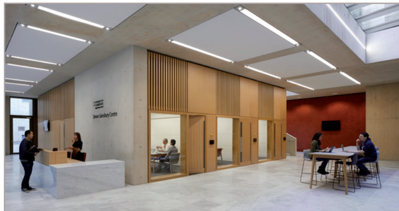
The Simon Sainsbury Centre, Cambridge used 50% GGBS in the mix for the project's extensive exposed concrete. The building achieved a BREEAM rating of Excellent. Image © Hufton and Crow.
